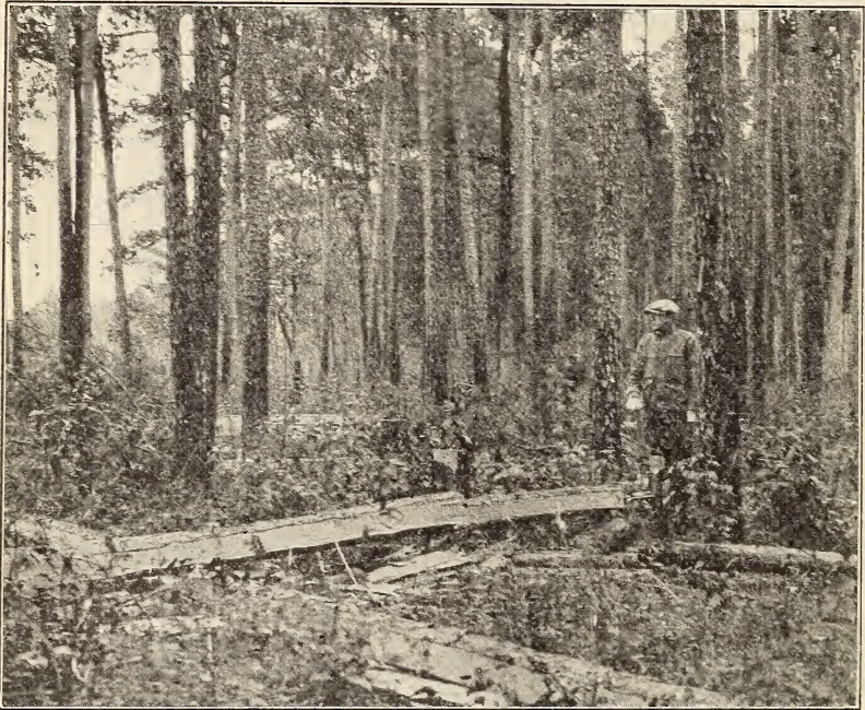
FIGURE 10.—In this tram-tie operation in second-growth loblolly and shortleaf pine in Louisiana the trees up to 10 inches are being hacked for ties; those over 10 inches will be cut into saw logs
